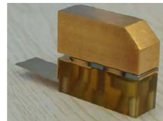
Figure 6 A sample of single-bar 250W QCW MaCC-packaged high power semiconductor laser array
