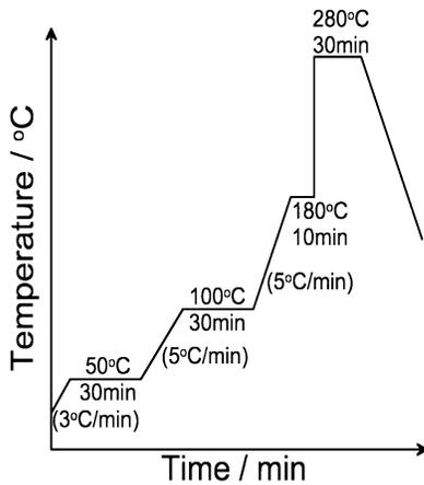
Fig.3. Low temperature sintering processing for nano-scale silver paste
