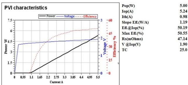
Fig.7. PVI curve of nano-scale silver paste packaged C-Mount semiconductor laser
