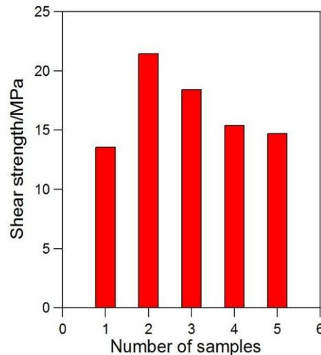
Fig.5. Shear strength distribution of nano-scale silver paste sintered C-Mount semiconductor laser
