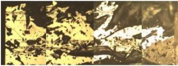
Fig.6. Failure section of chip inter plane separation
