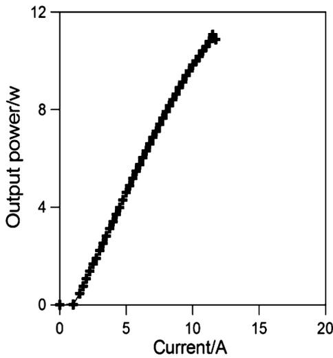
Fig.10. Thermal rollover of the device
