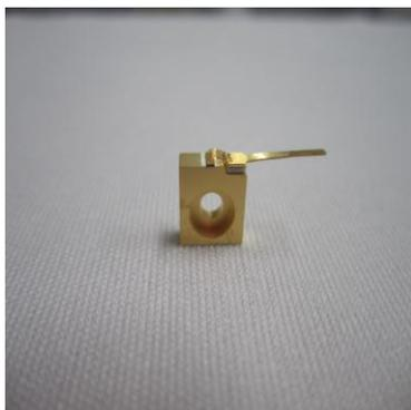
Fig.4. C-Mount semiconductor laser packaged with nano-scale silver paste
