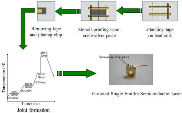
Fig.2. Preparation process of C-Mount laser diode
