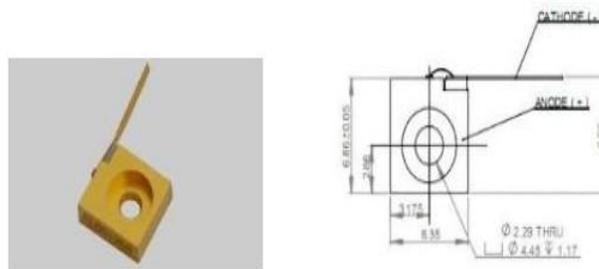
Fig.1. Structure of C-Mount semiconductor laser
