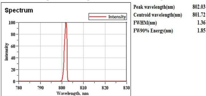
Fig.8. Spectral sweep result of nano-scale silver paste packaged C-Mount semiconductor laser
