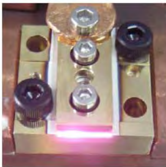
Figure 5 Example of the LIV testing of a single-bar 250W QCW conduction-cooled-packaged high power semiconductor laser array operating in high duty cycle (8%, 400Hz, 200μs)
